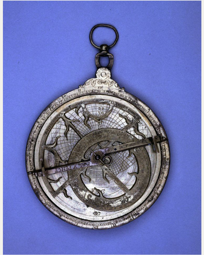
Henry VIII's Astrolabe made for the king by Bastien le Seney, the Royal Clockmaker, c.1545 [now in the British Museum]. An astrolabe was a primitive computer for calculating star positions.
